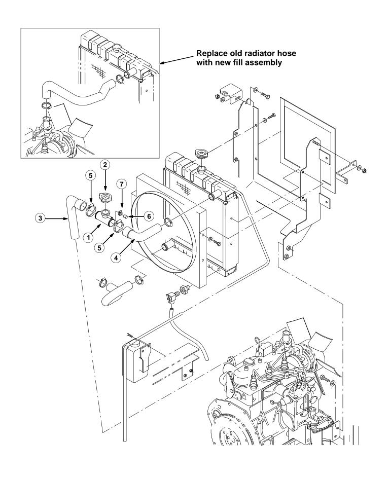
FIG. 1 - REMOTE FILL RADIATOR KIT INSTALLATION
